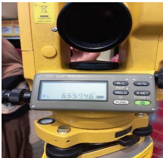
Figure 4: Theodolite Rotation Result According to the Qibla Azimuth
