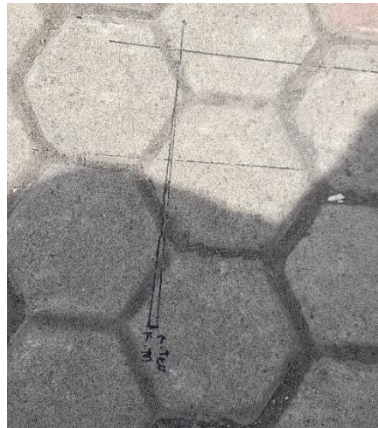
Figure 5: Deviation Result After Targeting Theodolite Points and Drawing the Shaf Line
